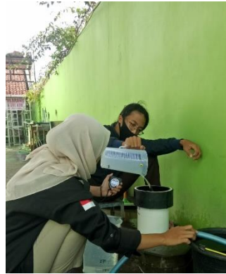
Gambar 3. Uji Infiltrasi Beton Porous
