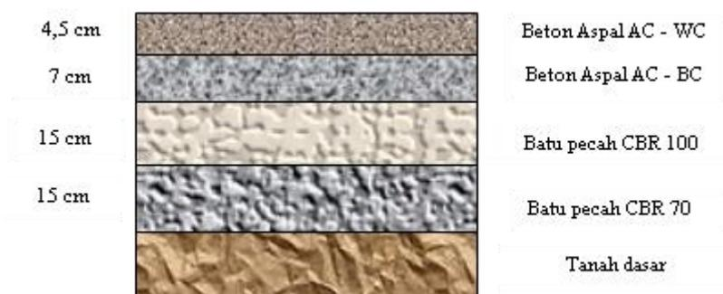
**Gambar 2.** Tebal Struktural Perkerasan Lentur Metode Pt T-01-2002-B
